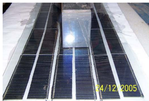
Figure 4: Capillarity encapsulated Evergreen String Ribbons during curing of the encapsulant.
