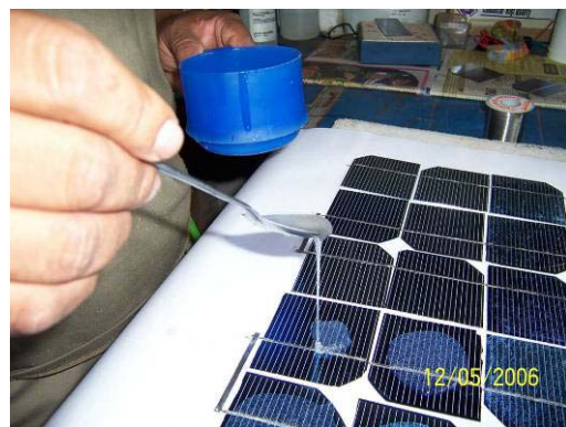
Figure 1: Dispensing of liquid silicone on top of the cells.
