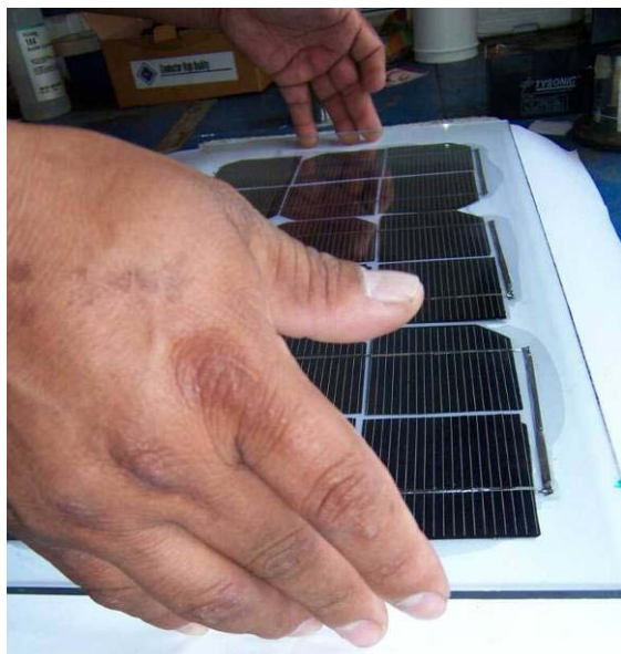
Figure 3: A standard window glass is positioned on top of the cells.
